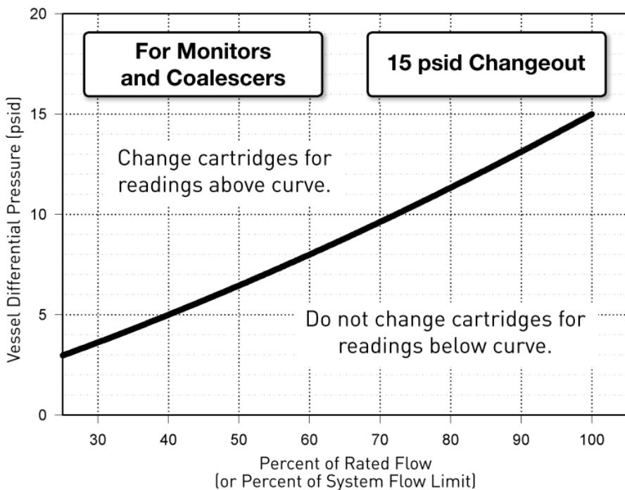
**EXAMPLE:** A 600 GPM vessel is operating at 300 GPM (50% of system flow limit). When the pressure differential reads less than 6.5 psid, the cartridges do not require changing. When the pressure differential reads 6.5 psid or more, or if the cartridges have been in service for one year, the cartridges are due for changeout.
